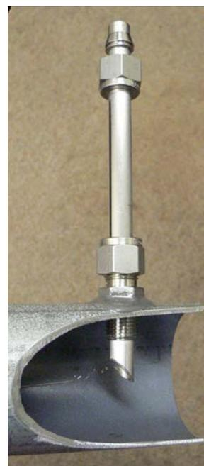
Swagelok Plug SS-600-P is used to cap the port when the probe is not installed. Alternatively, a short probe can be left in place and capped with a Swagelok SS-600-C.
